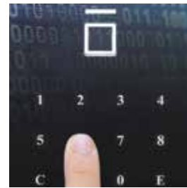
Anti-Peeping Password Scrambling Allows Entering Up To 30 Random Digits With The PIN Code To Confuse Onlookers
