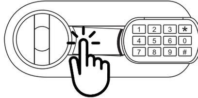
2. Insert emergency key into key access and turn key counter-clockwise. Hold the key to open position and turn the knob clockwise to open the door.
