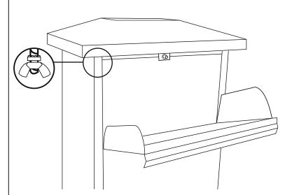
2 With drop slot open, screw in washer and bolt on to the screw to secure the roof to the parcel box. Repeat three more times with remaining screws.
