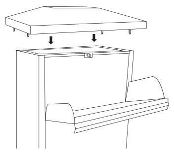
1 Place screws of the roof through the roof holes of the parcel box.
